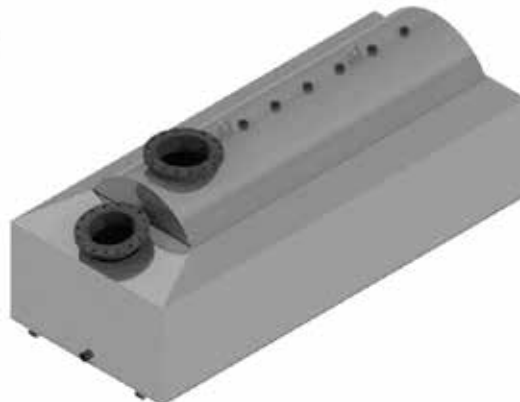
Cylindrical Tank with Containment
